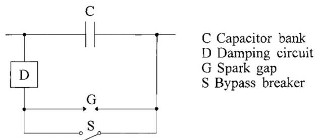
*Figure 2-4: Series Capacitor Scheme*
