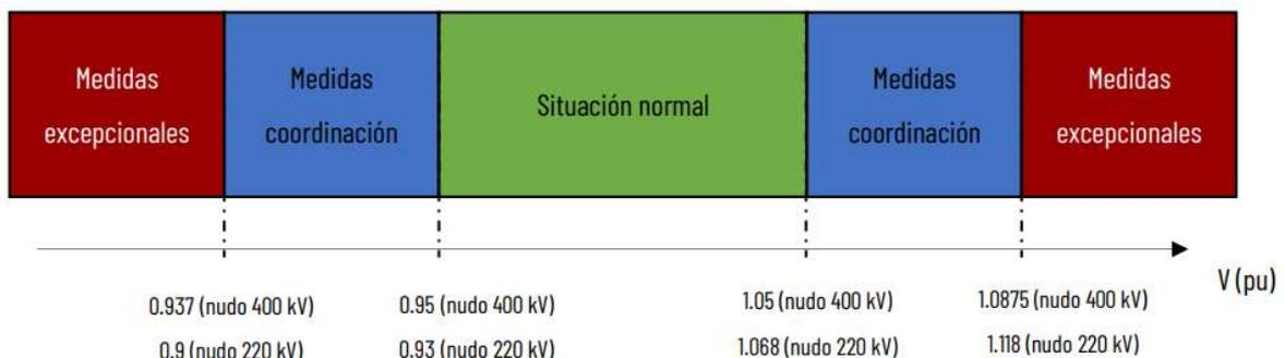
*Figure 4-1: Transformers operational range*
