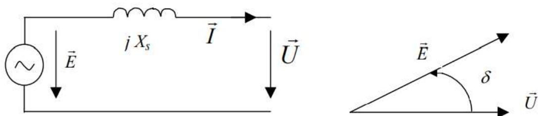
*Figure 3-4: Synchronous Machine Scheme[18]*
