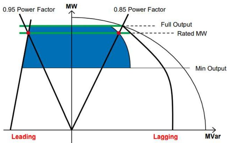
*Figure 4-4: Synchronous Generators operational requirements*
