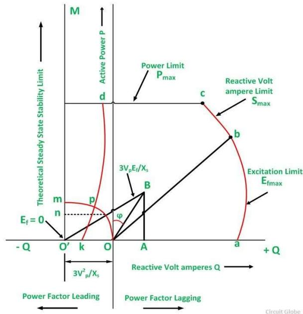
Figure 3-5: Synchronous Machine Operational Curve (Abacus P-Q)[19]
