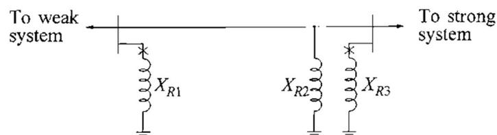
$X_{R2}$  – permanently line-connected reactor
