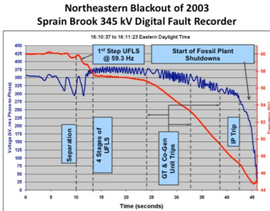
Figure 1-1: Voltage & Frequency Drop, Blackout 2003[2]
