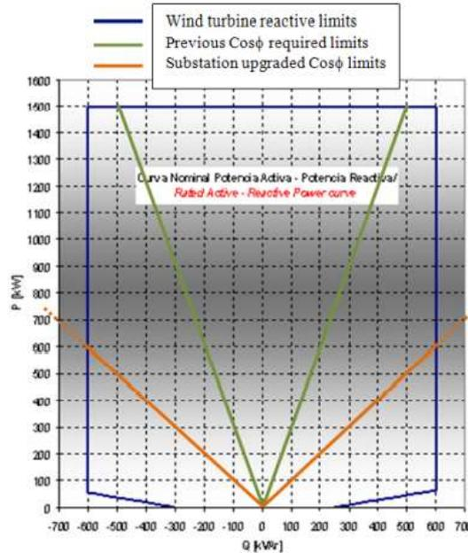
Figure 3-2: Reactive Power Limits in DFIG[14]
