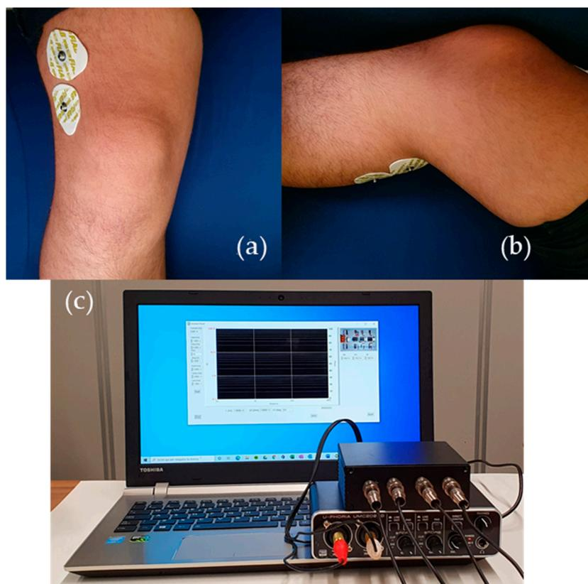
**Figure 9.** Electrodes arrangement (a) and (b) and developed measurement system (c).
