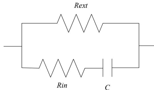
**Figure 3.** Equivalent circuit of a knee.  $R_{ext}$  models the extracellular liquids,  $R_{int}$  the intracellular liquids and  $C$  the capacitance of the cellular membrane.
