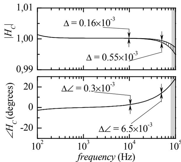
**Figure 4.** Modulus and the phase of the correction functions. The deviation is so small that the limiting curves can be distinguished, with the scale used for the figure, only in the case of the modulus and only for frequencies above 20 kHz.
