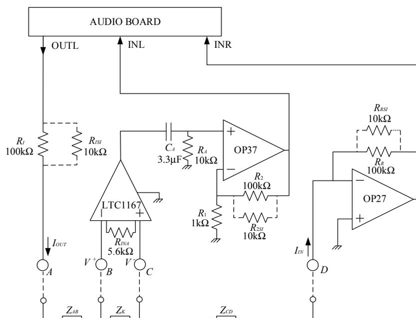
**Figure 1.** Circuit schematic of the proposed system.  $Z_k$  is the impedance of the knee, and  $Z_{AB}$  and  $Z_{CD}$  are the parasitic impedances between electrodes A and B and C and D, respectively.
