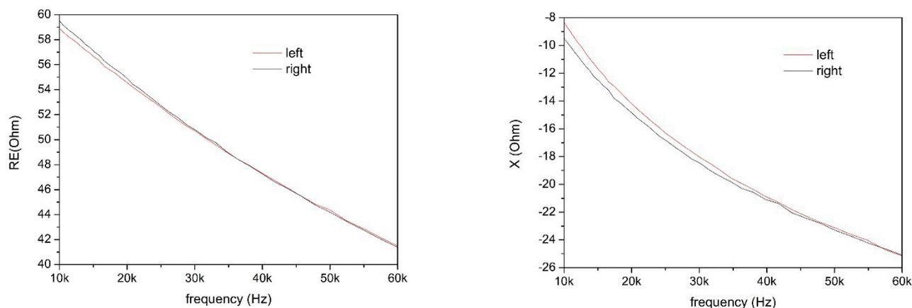
**Figure 10.** Resistance and reactance of the bioimpedance of subject S3 vs. frequency.
