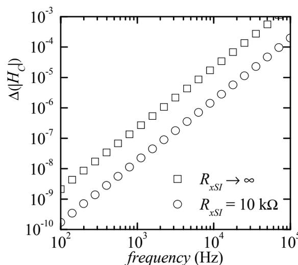
**Figure 5.** Maximum deviation of the modulus of the correction function  $H_c$  vs. frequency. The empty squares refer to the same simulation condition in which Figure 4 has been obtained. In the case of the empty circles, the only change was the presence of 10 k $\Omega$  snap-in resistances in parallel to  $R_L$ ,  $R_2$  and  $R_R$  in Figure 1.
