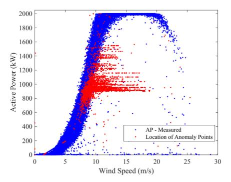
Figure 3. Anomaly detection capability in RCA methodology
