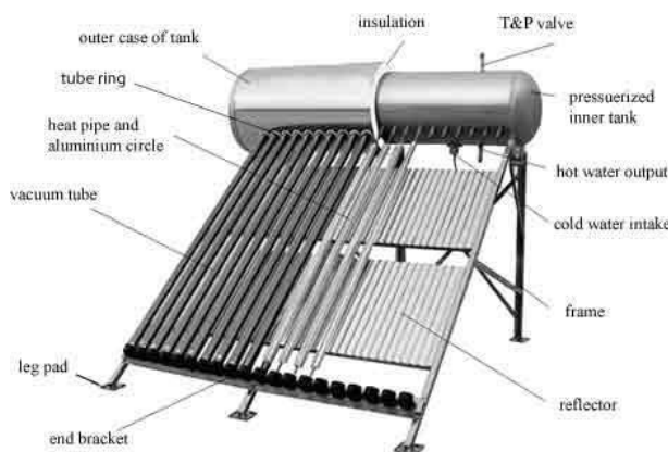
Figure 2. Schematic of a vacuum tube solar collector.[5]
