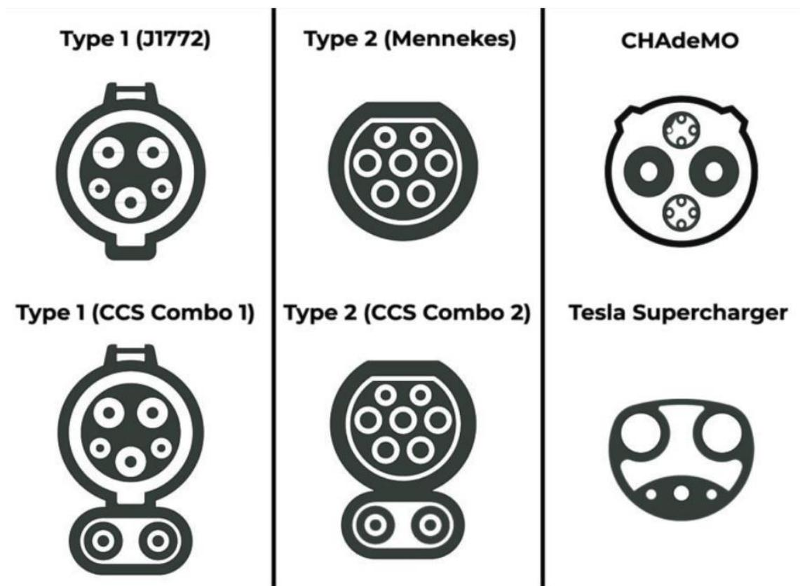
Figure 14. Main types of EV chargers. Source: [28]
