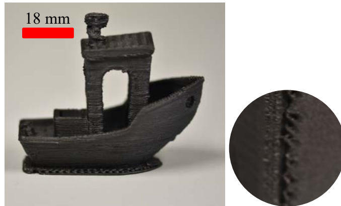
Figure 26. First 3DBenchy printed with CF-PEKK
