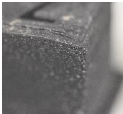
Figure 51. Warping experienced by the CF-PEKK calibration cube during annealing
