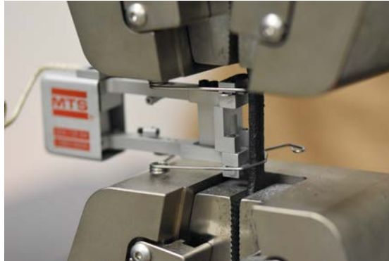
Figure 37. CF-PEKK coupon, held by the jaws of the tensile machine, with the extensometer placed in the gauge section
