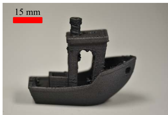
Figure 27. 3DBenchy printed with Kimya filaments following the optimal parameters, listed in Table 5
