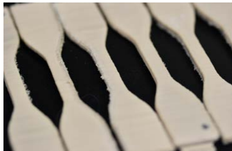
Figure 38. PEKK tensile coupons once annealed
