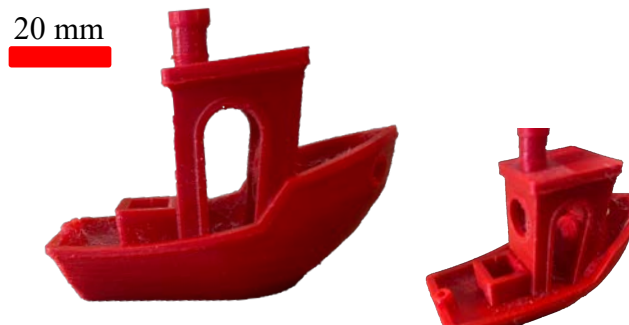
Figure 16. 3DBenchy printed with PLA optimal parameters
