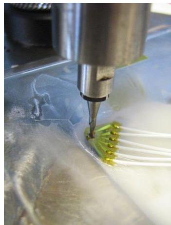
Figura 3.3, Hole Drilling, adaptado de HBM
