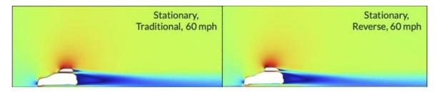
Figura 5: Velocity fields Traditional vs Reversed
