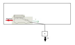
Figure 40:Scheme of the Wind tunnel procedure
