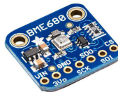
Figure 2.1: Humidity, temperature and altitude sensor BME 680
