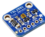
Figure 2.4: Light luminosity Lux sensor TSL2591
