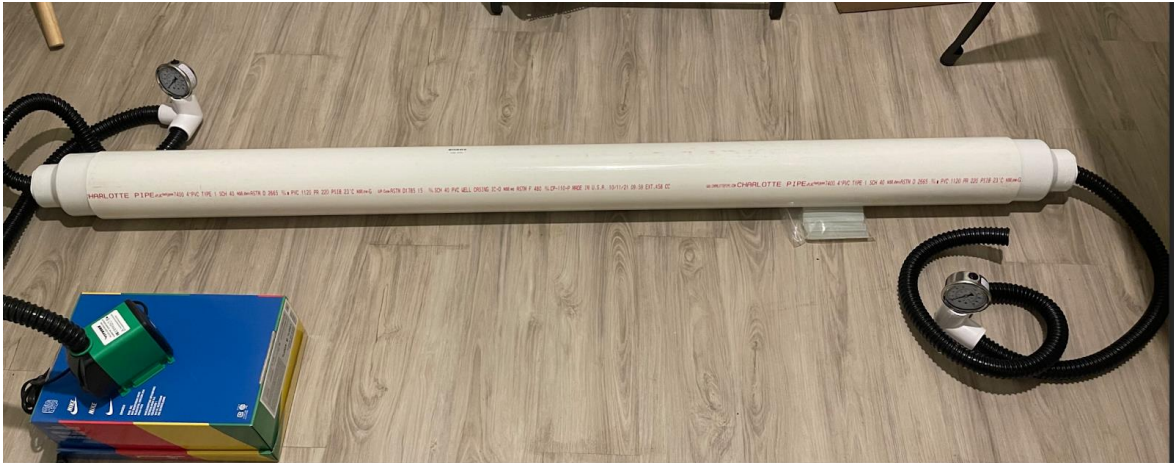
Figure 40. Pressure test set up
