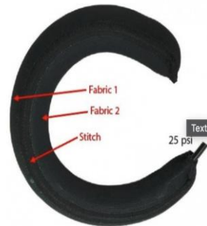
Figure 17. Pneumatic actuator design [3]
