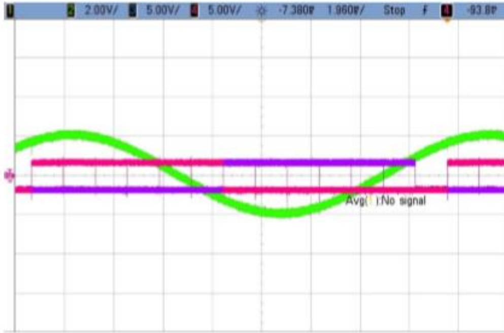
Figure 12: Output signal of microcontroller for MOSFET gate controls
