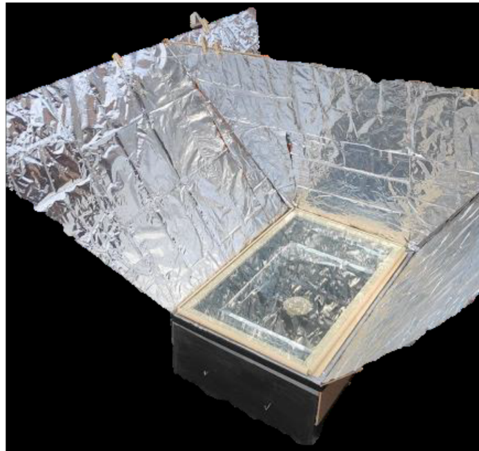
Figure 1. Prototype of solar oven built with recycled materials.
