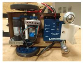
(b) Eve's underside, and engine assembly
