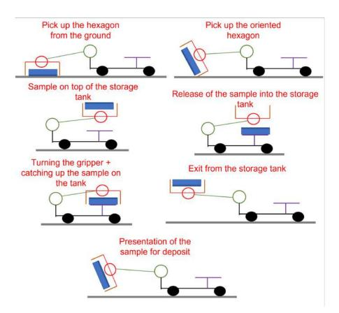
Figure 24: Sample of how the robot works
