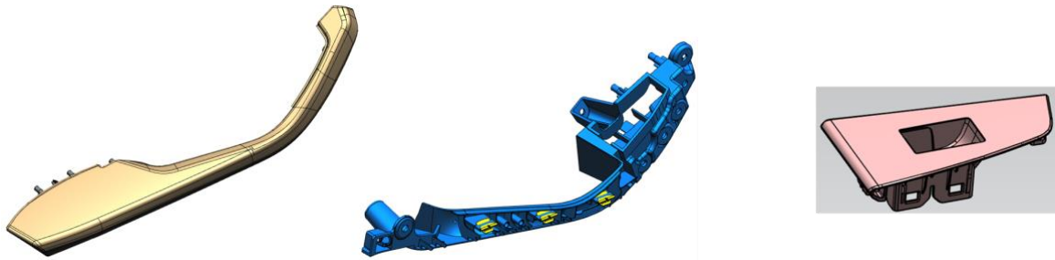
Figure 19 – BMW F7x Armrest, Grab Handle & Rear Switch Bezel (from left to right)
