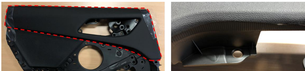
Figure 30 – BMW F7x Beltline covered with ESL and edge wrapped on the right
