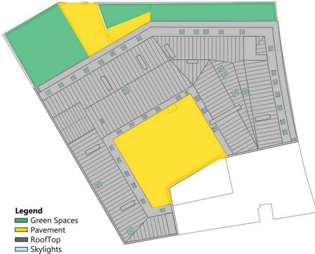
FIGURE 28 – HORIZONTAL SURFACE DIVISION BEFORE RENOVATION (SOURCE: PAYET)
