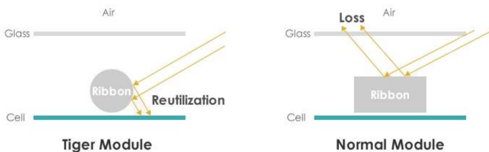
Figura 24 Comparación Ribbon circular vs. Ribbon rectangular [JINK20]
