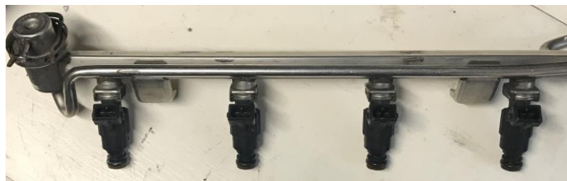
Illustration 7: Fuel rail with injectors and pressure regulator
