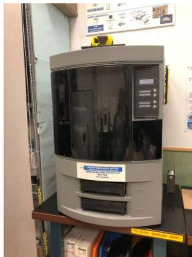
*Figura 26: Impresora Dimension SST 768.*
