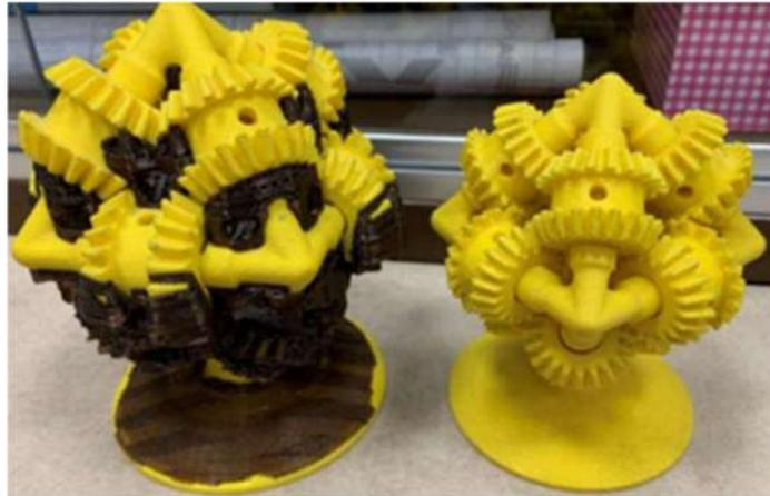
*Figure 7: Example from the ICAI laboratory of the before and after removal of the support material using the ultrasonic tank.*
