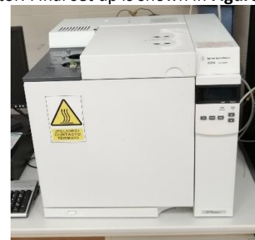
Figure 14. Agilent GC 7820A. Source: Own.
