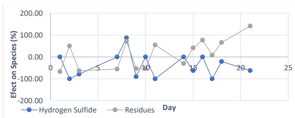
Figure 28: Effect of Nanoparticles on Hydrogen Sulphide and Residues in Batch Reactor. Source: Own.
