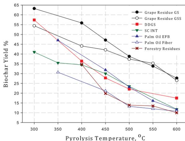
**Figure 4.** Effects of pyrolysis temperature on the biochar yield from various biomass residues, wt. % feed, at 5s vapor residence time [43]. GS (Grape Skins), GSS (Grape Skin and Seeds), DDGS (Dried Distiller's Grains), SC INT (Sugar Cane Internal Bagasse), EFB (Empty Fruit Bunches).
