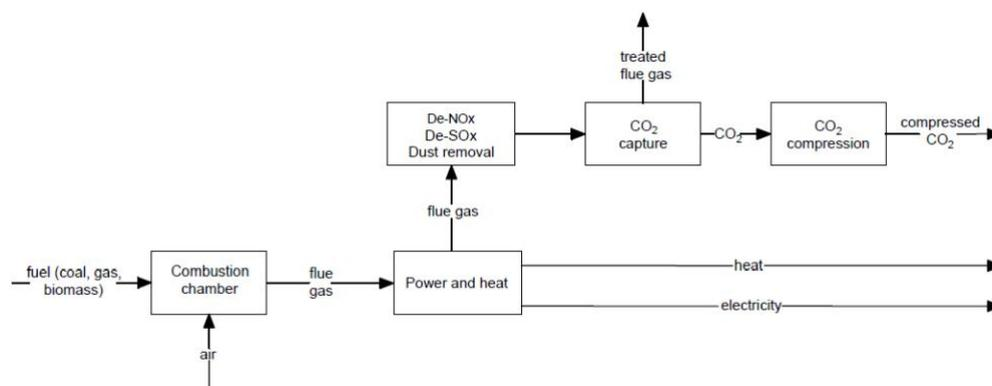
**Figure 8.** Post-combustion CO<sub>2</sub> capture process [68].
