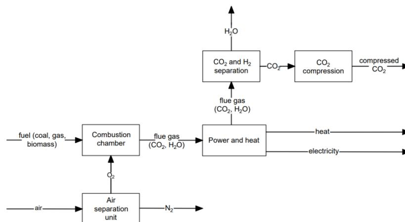
**Figure 10.** Oxy-combustion  $CO_2$  capture process [68].
