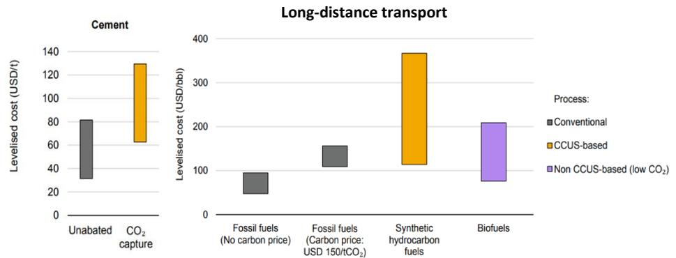
**Figure 12.** Simplified levelized cost of producing low-carbon cement and long-distance transport [91].
