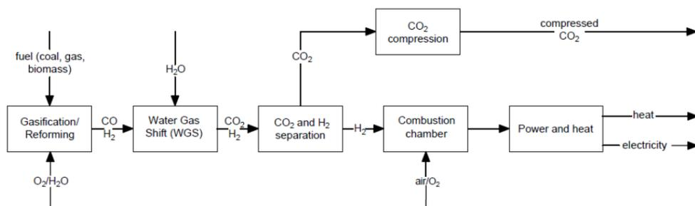
Figure 9. Pre-combustion CO<sub>2</sub> capture process [68].
