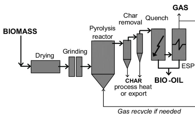
**Figure 3.** Simplified biomass pyrolysis process [37].
