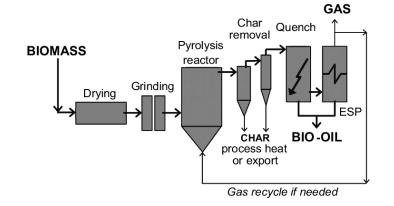
Figure 3. Simplified biomass pyrolysis process [37].
