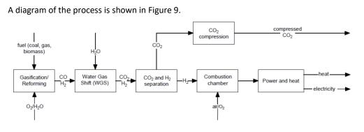
Figure 9. Pre-combustion CO2 capture process [68].
