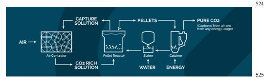
Figure 11. Chemical carbon removal process [86].
