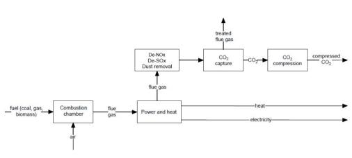
Figure 8. Post-combustion CO2 capture process [68].
