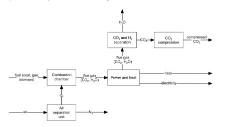
Figure 10. Oxy-combustion CO2 capture process [68].
