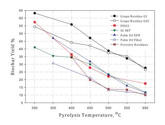
*Figure 4.* Effects of pyrolysis temperature on the biochar yield from various biomass residues, wt. % feed, at 5s vapor residence time [43]. GS (Grape Skins), GSS (Grape Skin and Seeds), DDGS (Dried Distiller's Grains), SC INT (Sugar Cane Internal Bagasse), EFB (Empty Fruit Bunches).
