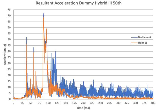
Figure 7: Resultant acceleration from Dummy Hybrid III simulations
