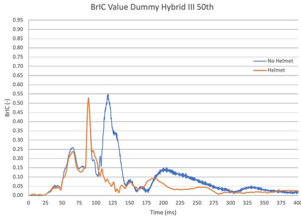
Figure 9: BrIC graph from Dummy Hybrid III simulations
