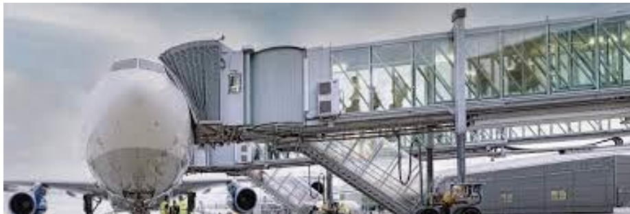
Fig 3.1. ThyssenKrupp’s TB 45/26.5-2 loading walkway.
