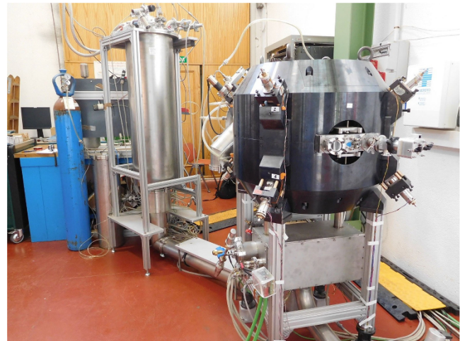
Fig. 1. AMIT superconducting cyclotron and the cryogenic supply system (CSS).
