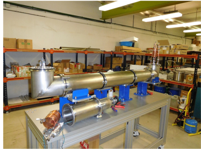
Fig. 3. Assembly of the new transfer line.
