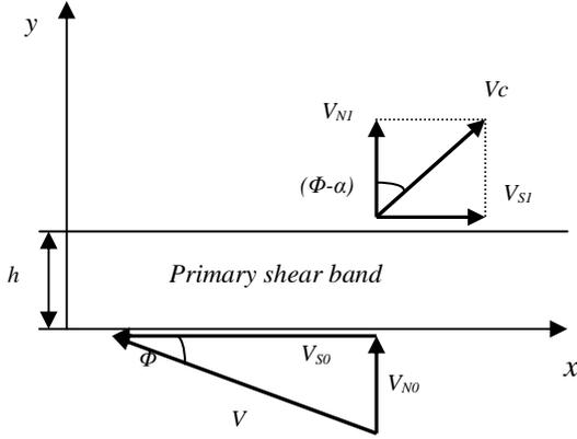
Fig. 1. Analytical modelling of orthogonal cutting, Molinari *et al.* [1992].
