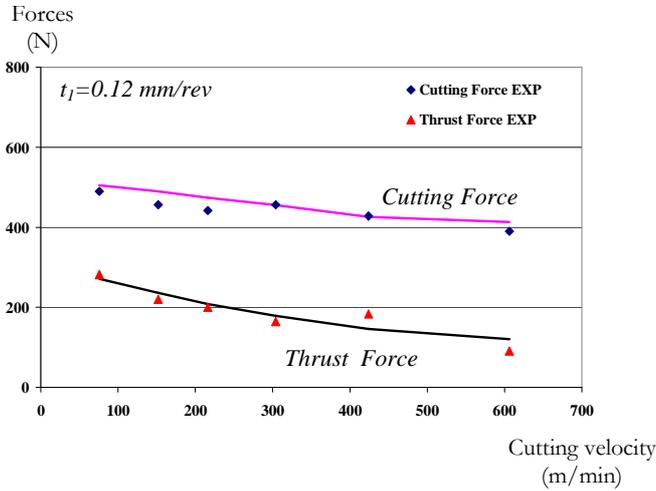
Fig. 2. Comparison between predicted (lines) and experimental data for the values of undeformed chip thickness. The cutting conditions are: the cutting angle  $\alpha = 5^\circ$ ,  $w = 2$ mm, feed = 0.12 mm/rev
