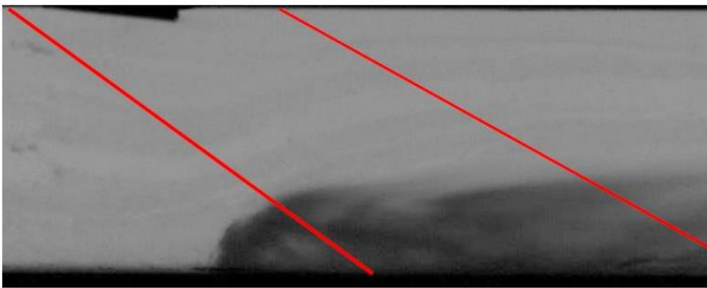
Image 14. Image showing the course of the supersonic waves.
