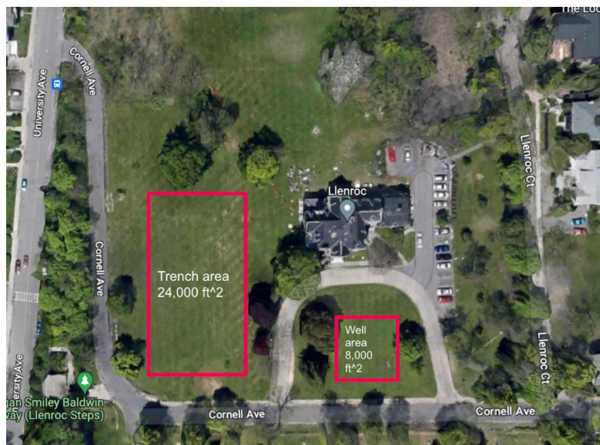
Figure 2: Areas of trenches and wells for the heat pump in Llenroc's yard
