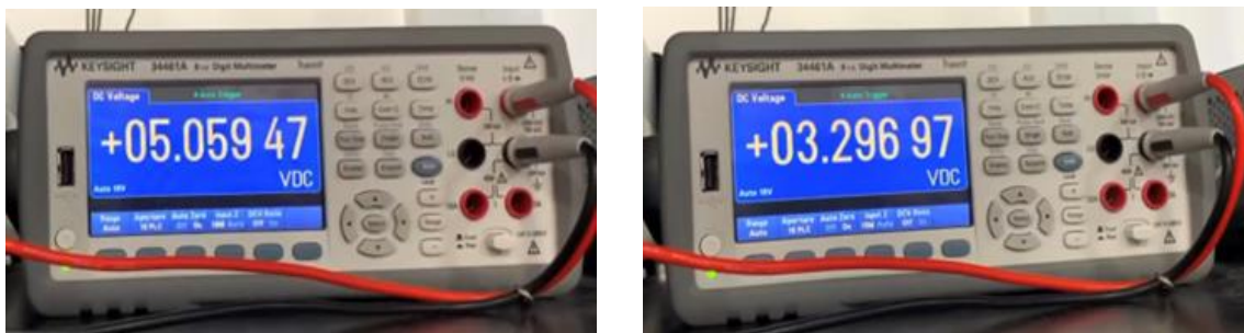
Figure 24. Output voltage of the 5V regulator (left) and the 3.3V regulator (right).
