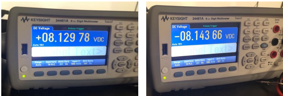
Figure 25. Battery voltages before (left) and after (right) charging the battery.
