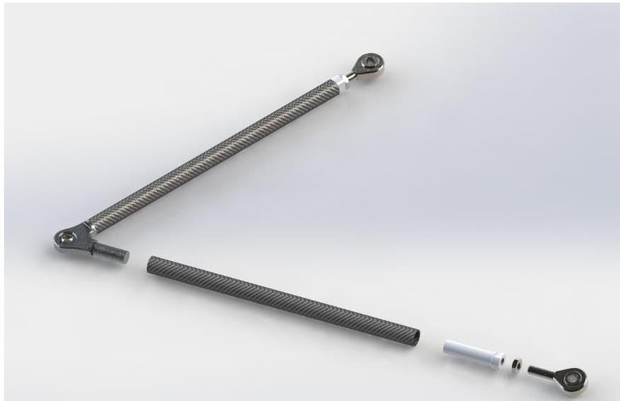
*Figure 45: Exploded view of a wishbone*
