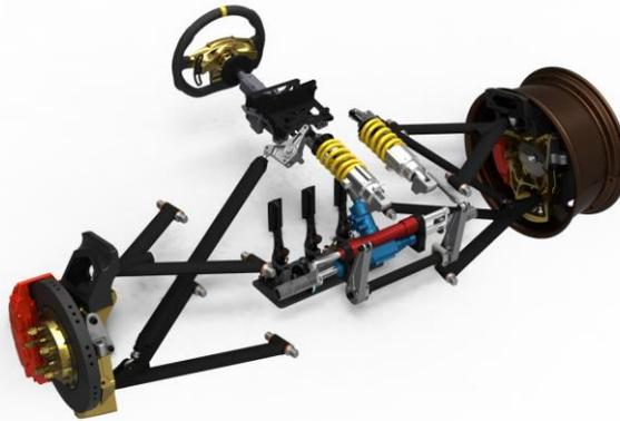
*Figure 12: Double wishbone suspension*
