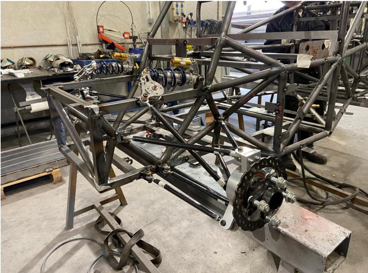
*Figure 57: rear suspension soldering*
