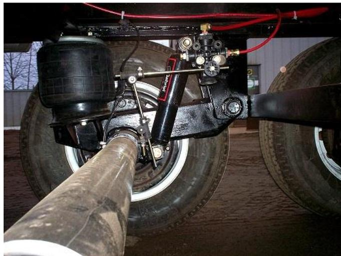
*Figure 14: Air Suspension*
