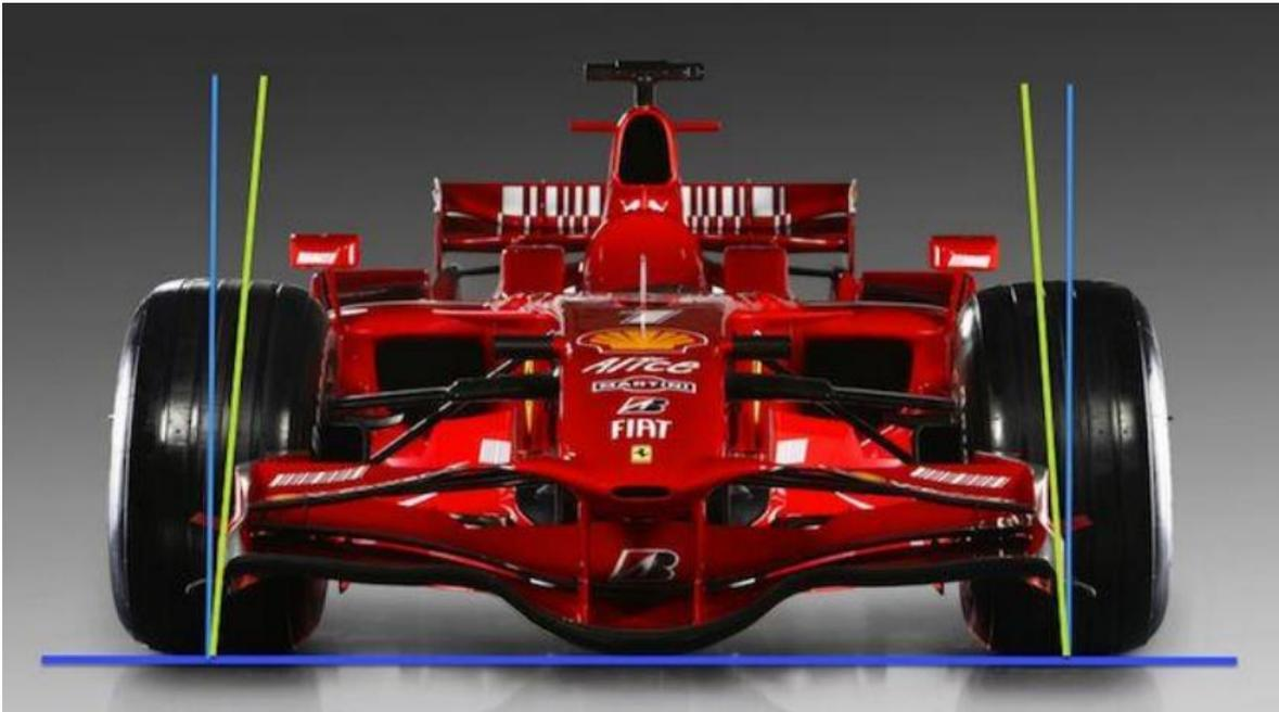
*Figure 18: Negative Camber angle in a Formula 1*
