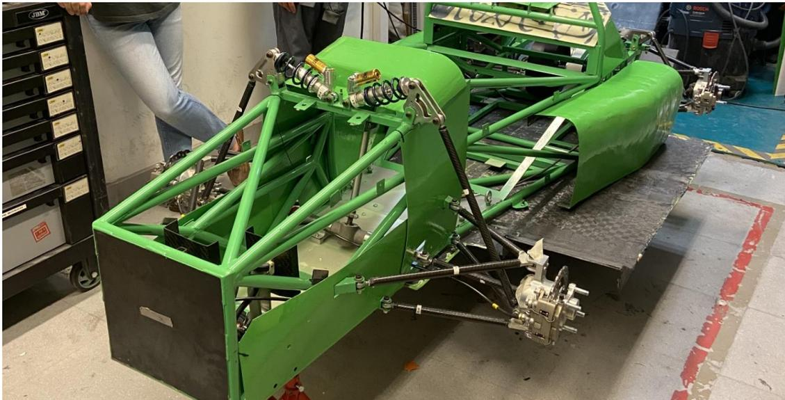
*Figure 8: Detail of the front suspension of the IFS04*
