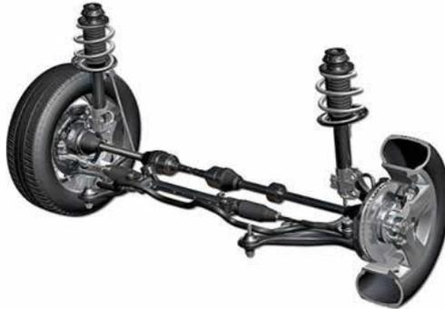
*Figure 11: McPherson suspension*
