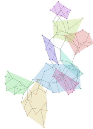
Fig 7. Example of Energy Community Detection using Quantum Computing for Simplifying a Meshed Network [17]
