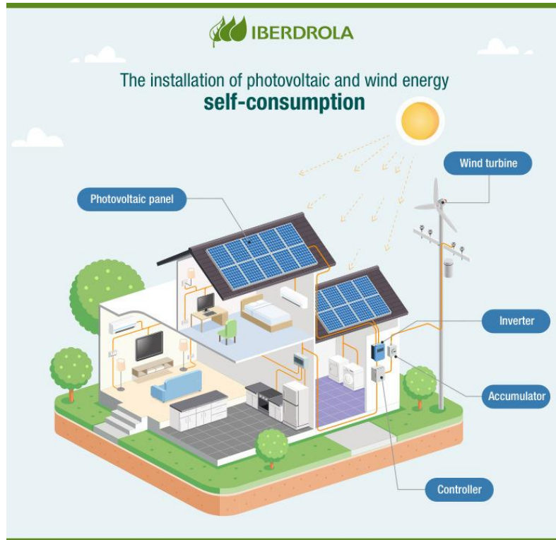
Figure 2: Installation of photovoltaic and wind energy self-consumption
