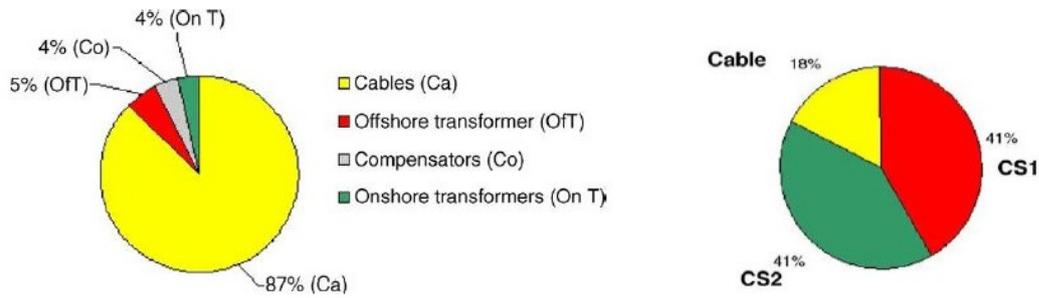
Figure 2.18: Participation of each transmission losses for 500 MW wind farm at 100 km transmission distance in HVAC (left) and HVDC (right). [23].
