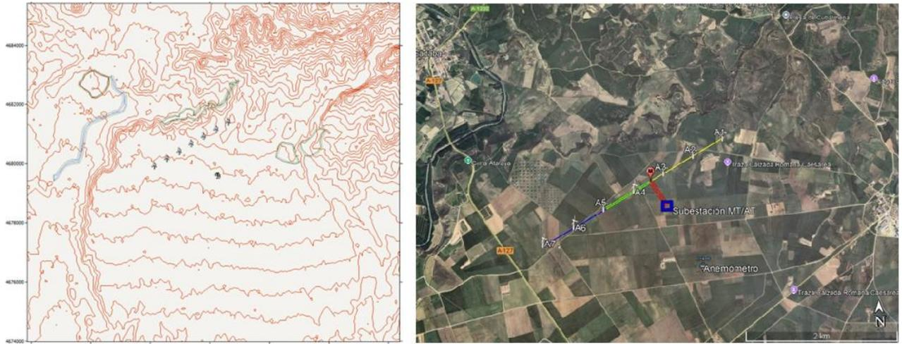
Illustration 4: Position of the wind farm on digitized topography and roughness map and detail of electrical infrastructure and generation circuits on site [WAsP, Google Earth Pro].
