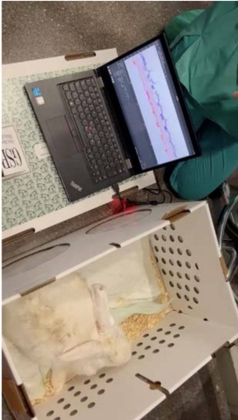
Figure 1.17: Image taken post-operation where the testing process can be seen taking place. The rabbit is encased in a box, while at the same time monitoring the prototype through the explained interfacing (Scopy and ADC). The image shows the instant that activation is recorded for the first time from the EMG capturing device. 18
