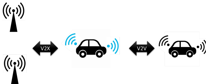
Figure 2.1: Vehicular networks simple representation of its main communications.
