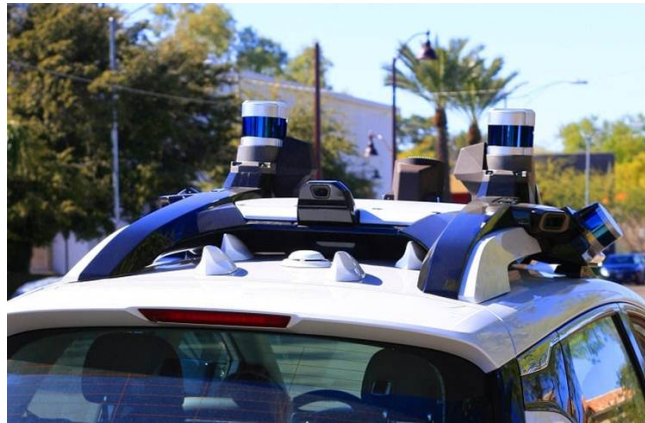
Figure 3.2: Example of hardware redundancy in AVs, picture from [18].
