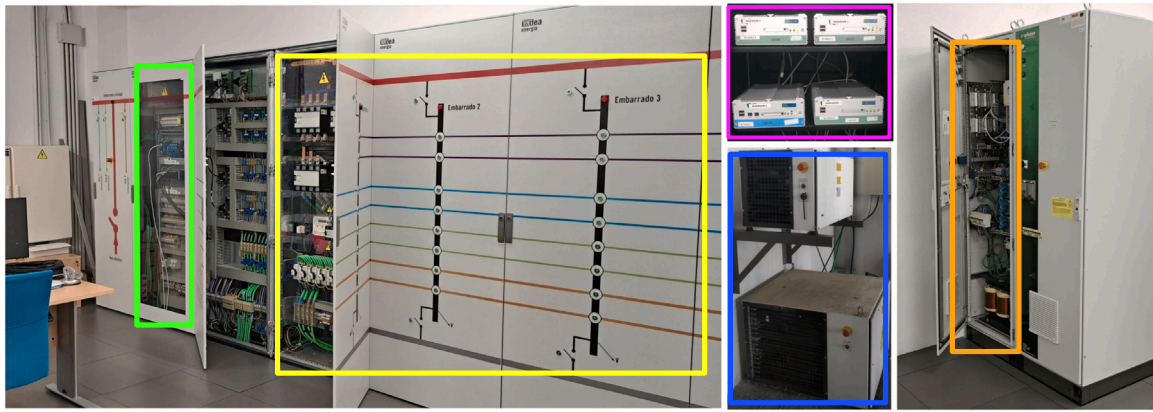
Fig. 11. Pictures of the laboratory facilities. (green) Centralised MG controller and measurements, (yellow) ac busbars, (violet) real-time computers, (blue) loads and (orange) power converters. (For interpretation of the references to colour in this figure legend, the reader is referred to the web version of this article.)
