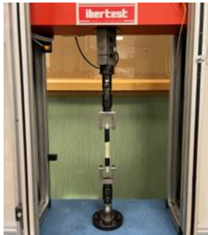
Figure 7 Suspension arm testing
