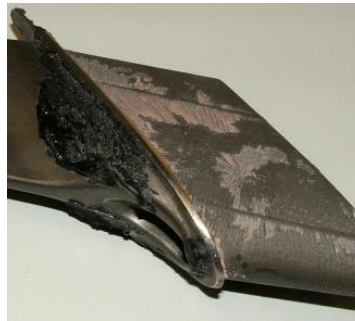
figure 26 Adhesive failure (SAVA10b) [10]
