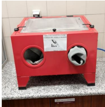
figure 32 Grit blasting machine used
