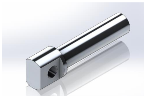
Figure 4 CAD view of the testing end-fitting model
