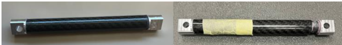
Figure 16 Testing end-fitting before (left) and after (right) testing
