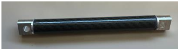
Figure 6 Suspension arm used for testing manufactured
