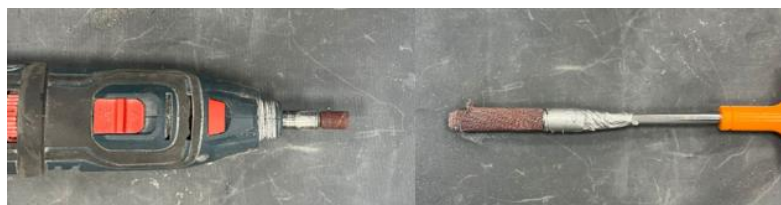
figure 31 Tools used for sanding the interior of the CFRP tube
