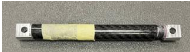
figure 77 Suspension arm before testing
