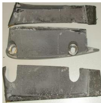
figure 27 Cohesive failure (SAVA10b) [10]
