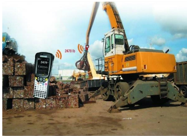
WIRELESS GRAPPLE SCALE ALLOWS SCRAP OPERATIONS TO ADD IN-MOTION WEIGH CAPACITY, RECYCLING PRODUCT NEWS
