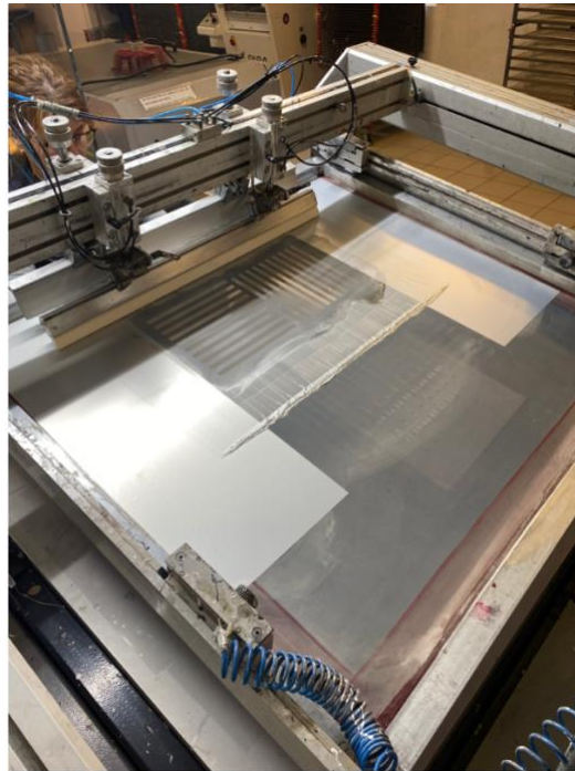
Figure 10: screen printing using silver ink
