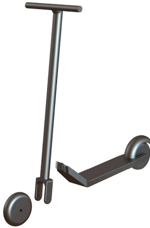
Fig. 2. Exploded view of e-scooter model: Parts 2, 1 and 3 (left to right).
