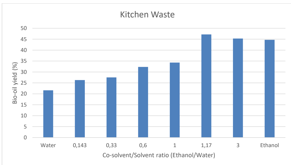
Graphic 12: Effect in kitchen waste liquefaction of co-solvent/solvent ratio in the bio-oil yield (%)
