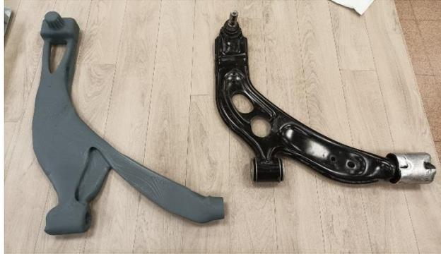
*Figure 15. Printed prototype using FDM technology, compared to the original component. (Author's own work)*
