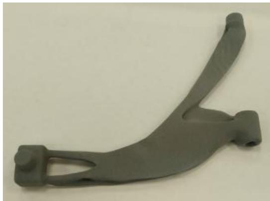
*Figure 16. Printed prototype using MJF technology. (Courtesy of Mariano Jiménez Calzado)*
