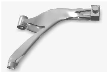
*Figura 13. Geometric modification of the Suspension Arm according to manufacturing criteria. (Author's own work)*
