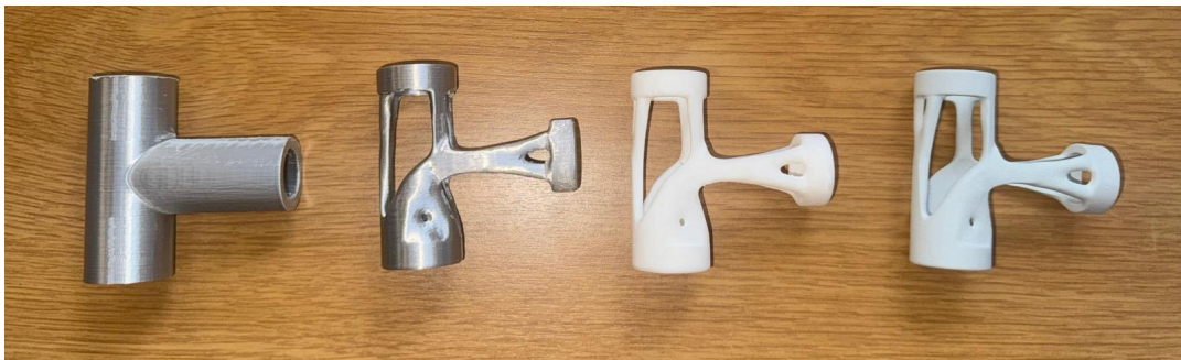
Ilustración 4. Visual comparison between the solid FDM-printed piece and the refined versions manufactured with FDM, SLA and MJF
