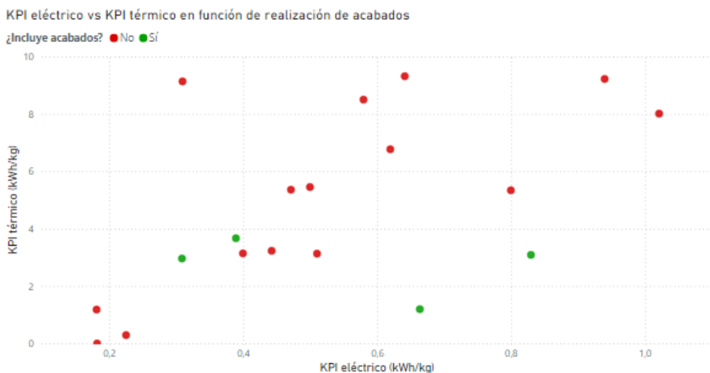
Figure 17. Electric and thermal KPI based on the inclusion of a finishing process
