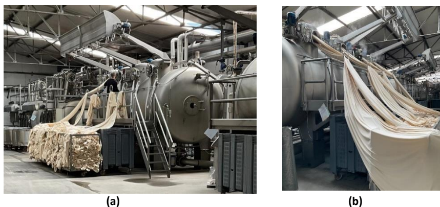
Image 3. Fabric dyeing machine during the loading process.
