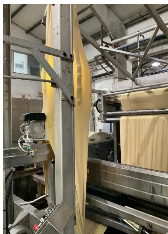
Image 6. Fabric dyeing machine pictures; (a) interior of the fabric dyeing machine; (b) descriptive diagram of its functioning. 312 313 314
