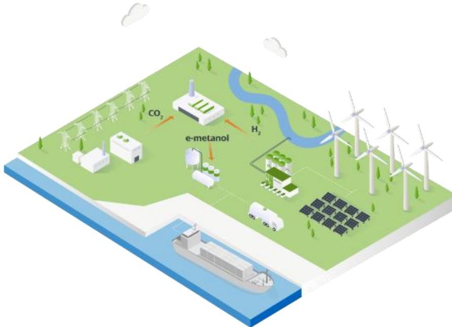
Image 2. Green Methanol Production System (Source: Iberdrola)
