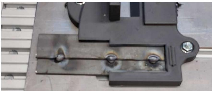
*Figura 5: Tack welding result in lap joint position.
