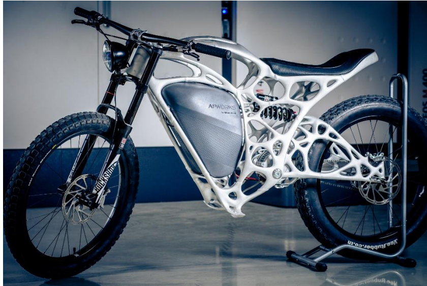
Ilustración 14 First 3D-printed Motorcycle by APWorks (Airbus Group) called Lightrider. https://www.altair.com/es/resource/apworks-light-rider-optimization-process
