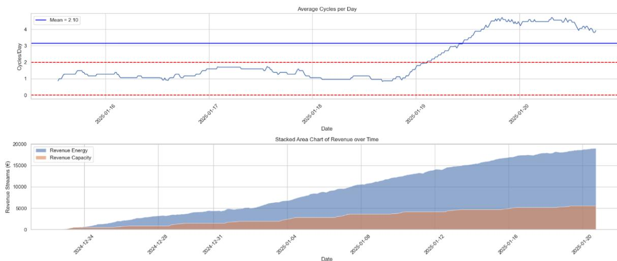
Figure 33: Monthly Revenue and Cycles per Day in the Capacity Auction in the Adaptive Strategy: Optimized Capacity and Price Premium Based on Previous 3 Days for 2h Battery
