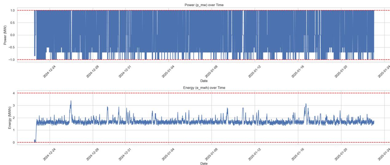
Figure 37: Power and Energy in the Adaptive Strategy: Hourly Optimized Capacity and Price Premium Based on the Previous Day for 4h Battery
