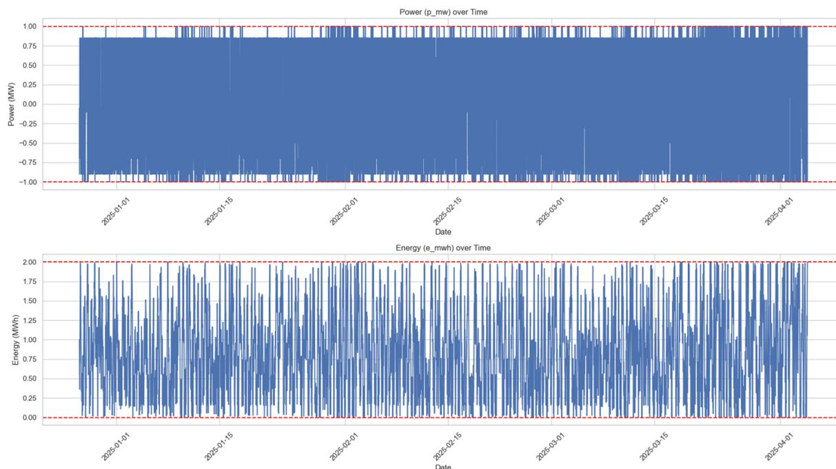
Figure 19: Power and Energy in the Deterministic Strategy: Energy-Only Optimization for 2h Battery
