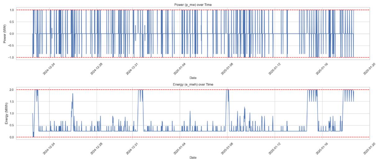
Figure 30: Power and Energy in the Adaptive Strategy: Optimized Capacity and Price Premium Based on Previous 3 Days for 2h Battery
