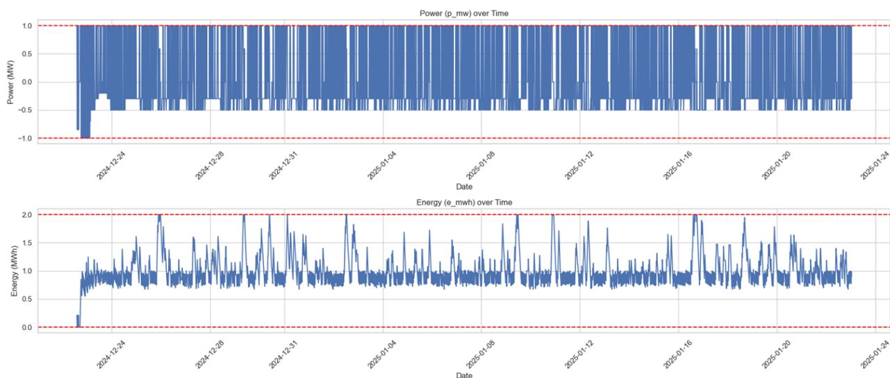
Figure 34: Power and Energy in the Adaptive Strategy: Hourly Optimized Capacity and Price Premium Based on the Previous Day for 2h Battery
