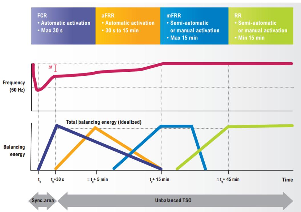
Figure 2: Balancing mechanism [17]
