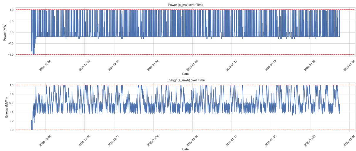
Figure 40: Power and Energy in the Adaptive Strategy: Hourly Optimized Capacity and Price Premium Based on the Previous Day for 2h Battery
