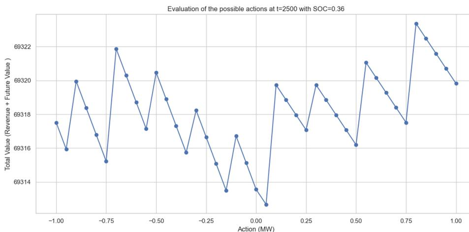
Figure 18: Evaluation of total value (immediate revenue plus future value) for all possible actions at time step  $t = 2500$ , given a state of charge (SOC) of 0.36. The action space corresponds to discrete power setpoints ranging from full discharge (-1 MW) to full charge (+1 MW). This plot illustrates how the dynamic programming algorithm assesses the optimal decision at a given state.
