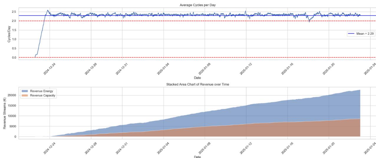
Figure 38: Cycles per day and Revenue in the Adaptive Strategy: Hourly Optimized Capacity and Price Premium Based on the Previous Day for 4h Battery
