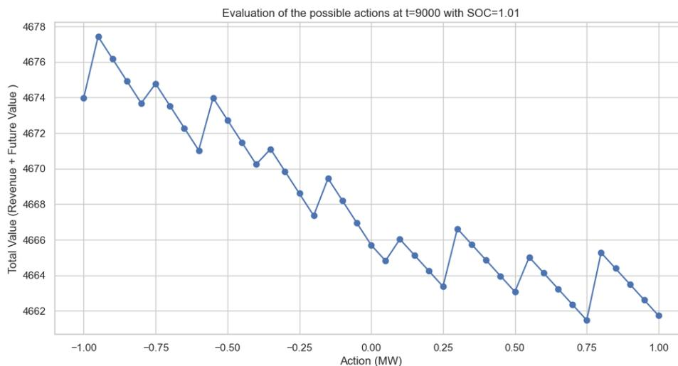
Figure 17: Evaluation of total value (immediate revenue plus future value) for all possible actions at time step  $t = 9000$ , given a state of charge (SOC) of 1.01. The action space corresponds to discrete power setpoints ranging from full discharge (-1 MW) to full charge (+1 MW). This plot illustrates how the dynamic programming algorithm assesses the optimal decision at a given state.
