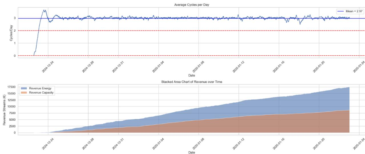
Figure 36: Cycles per day and Revenue in the Adaptive Strategy: Hourly Optimized Capacity and Price Premium Based on the Previous Day for 2h Battery
