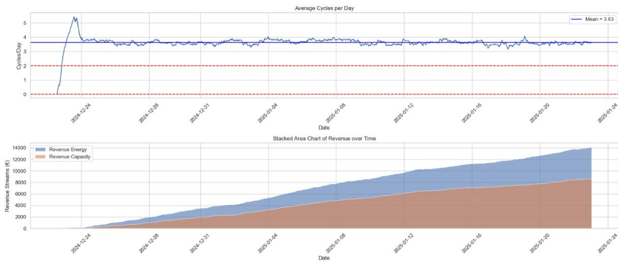
Figure 39: Cycles per Day and Revenue in the Adaptive Strategy: Hourly Optimized Capacity and Price Premium Based on the Previous Day for 1h Battery
