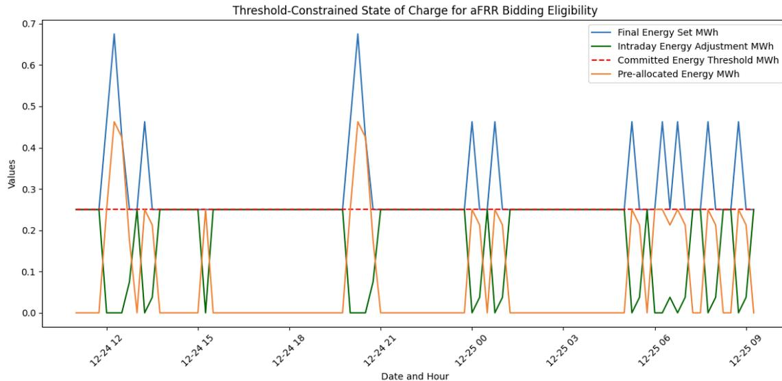
Figure 4: Threshold-Constrained State of Charge for aFRR Bidding Eligibility
