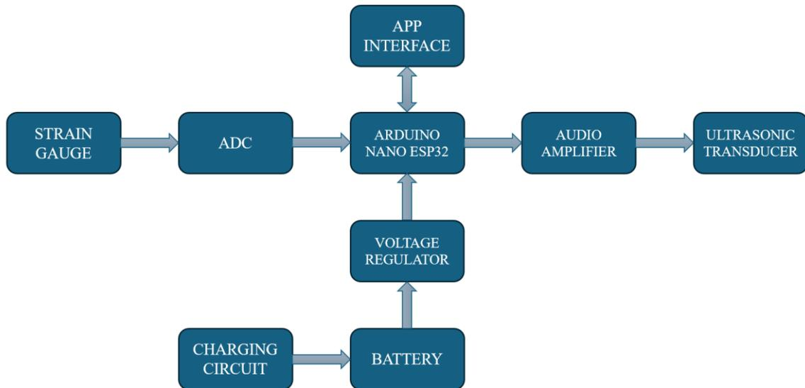
Image 8 - System block diagram
