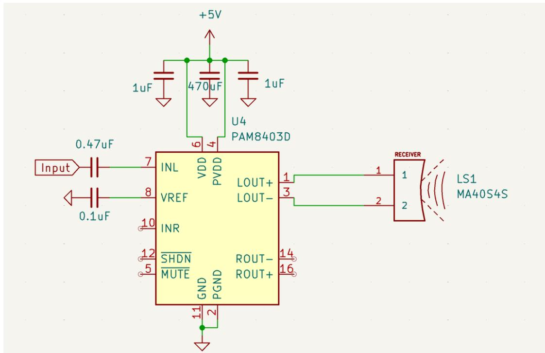
Image 7 - Corrective sound emission subsystem
