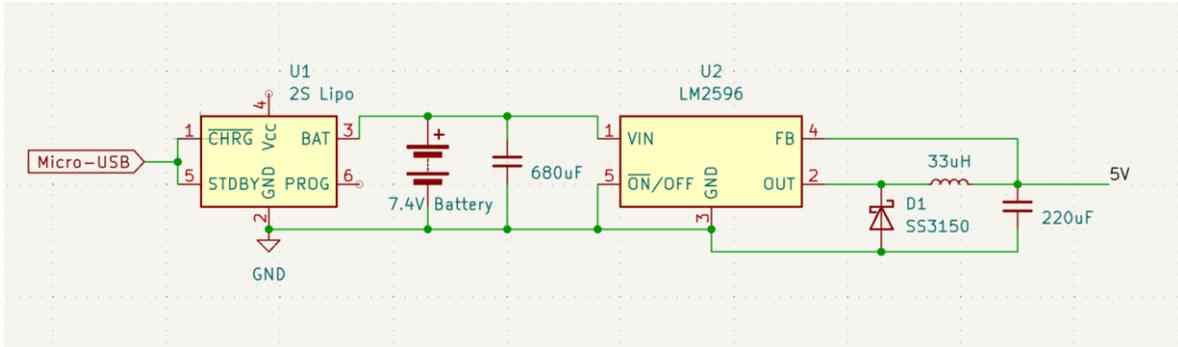
*Image 6 - Power supply circuit*
