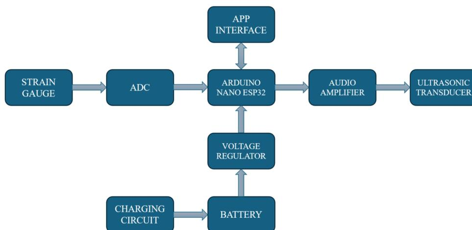
Image 3 – Collar’s system block diagram
