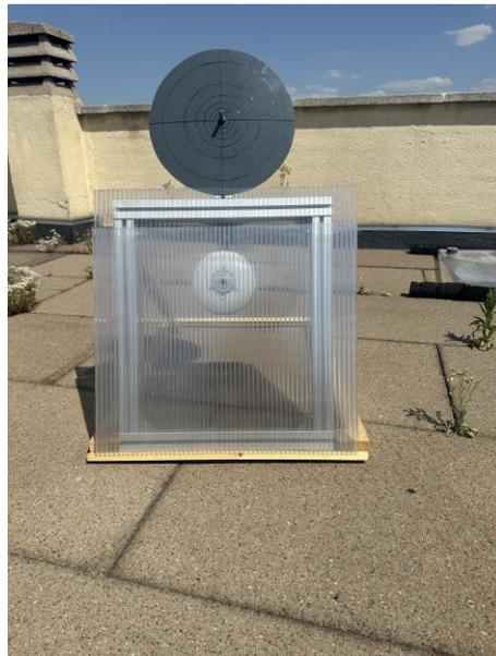
*Figure 2. Frontal view of the structure with double panel with the channels of the most exposed one in a vertical arrangement.*
