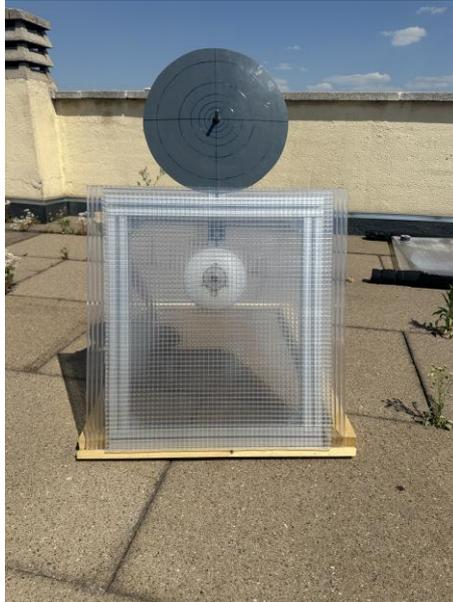
*Figure 3. Frontal view of the structure with double panel with the channels of the most exposed one in a horizontal arrangement.*
