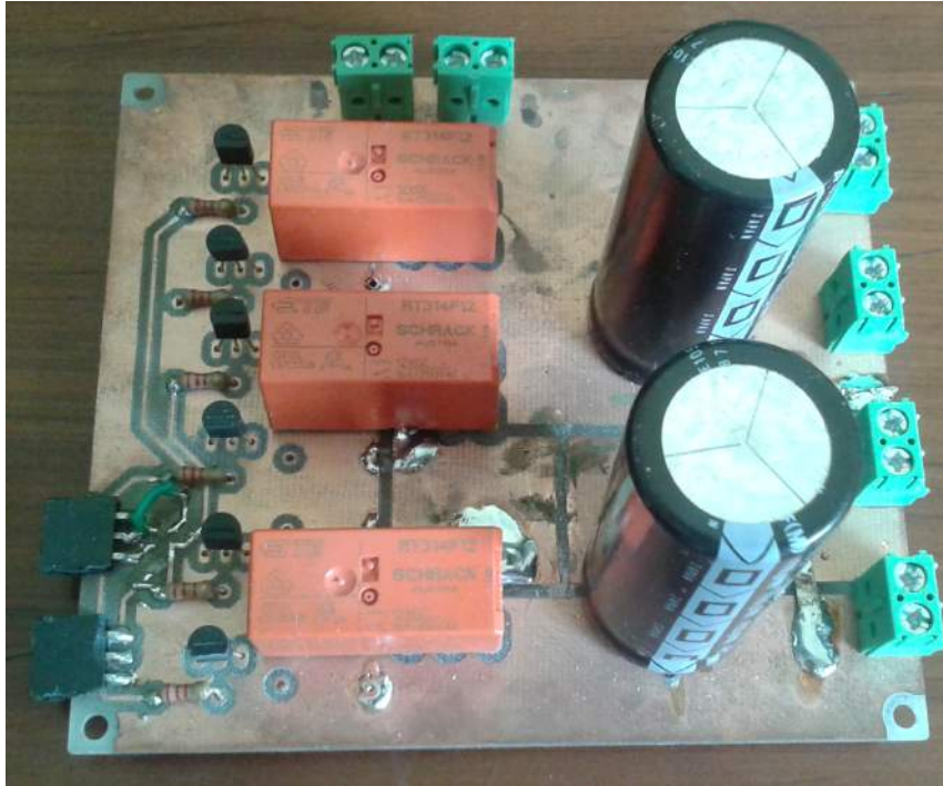
Figure 40. Manufactured and Assembled Relay PCB
