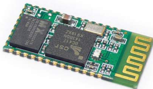
Figure 21. HC-05 Bluetooth Module
